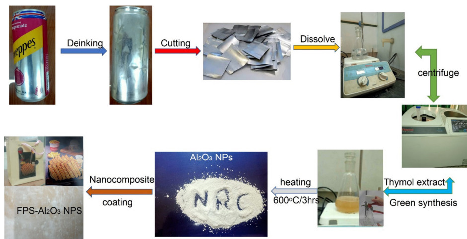
SCHEME 1 | Schematic diagram of FPS- \text{Al}_2\text{O}_3 -NPs green synthesis.
